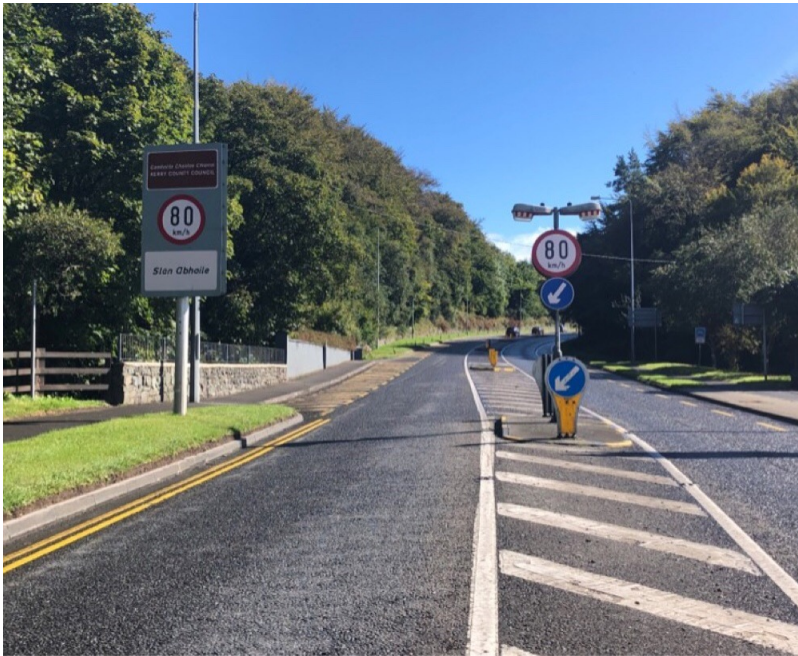
Location 37 - Splitter Island Numerous After Roundabout Direction Continue On N22 Visual inspection indicates that loaded blade will navigate this spiller island without issue *Note* Road width - 4.5
